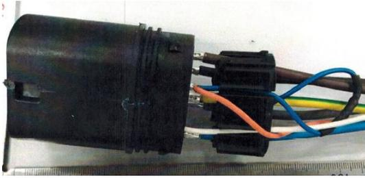
4. Push the piece at point 1 until you hear a click. Once fitted, it cannot be removed again.
