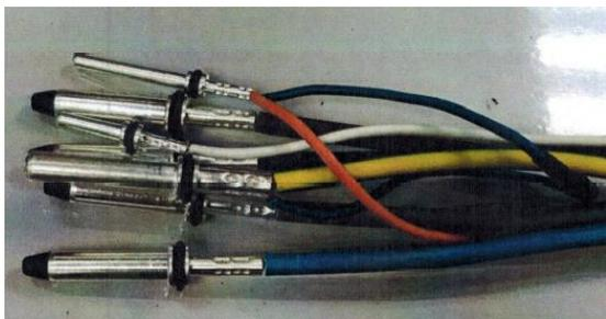
2. Pass the cables through the connector security piece
